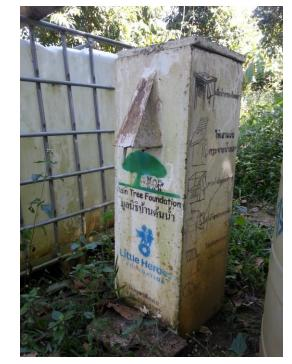
About 12 to 18 liters of clean water can be obtained (maximum capacity 150 liters a day). Any kind of water can be used in the BioSand Filter, well water, borehole water, pond or river water, tap-stand water or rainwater.
