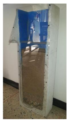
through the sand and then the gravel and conducted through an outlet tube.
